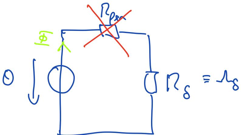
$$R_s = R_{air} = \int_l \frac{dl}{\mu \cdot S} = \frac{l}{\mu \cdot S}$$
